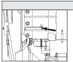
Chain Sprocket Shaft - 1 Zerk
