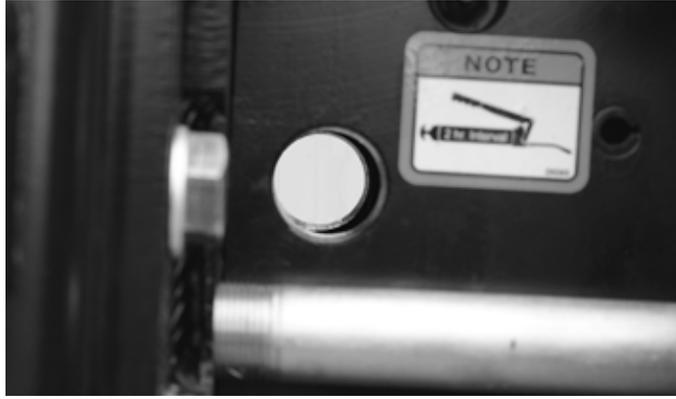
STEP 10: Have the helper reinstall the large retention pin with the groove oriented to the right of the Hornet. (When the large retention pin is properly installed, the ends of the pin will be flush with the power cell on both sides.)
