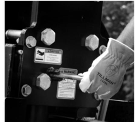
STEP 4: Have the helper remove the large retention pin from the right side of the Hornet. Use the smaller retention pin to push the larger retention pin out until it can be grasped and pulled by hand. If the driving tool is properly supported, the large retention pin should slide out with ease.
