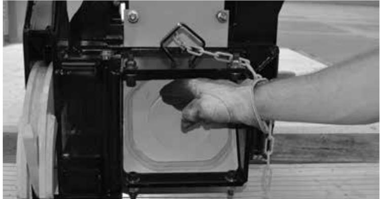
STEP 9: Using the vehicle, slowly tilt the Hammer to the upright position. Once the weight begins to slide down the Hammer case, momentarily stop tilting the Hammer so the weight can slowly slide to the bottom of the case.
