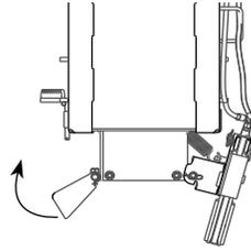
STEP 3: Route the hydraulic hoses through the quick attach plate hose holder, and connect the hydraulic hoses to the vehicle's auxiliary hydraulics.
