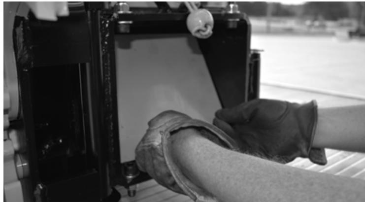
STEP 10: Using the vehicle, slowly tilt the Hammer to the upright position. Once the weight begins to slide down the Hammer case, momentarily stop tilting the Hammer so the weight can slowly slide to the bottom of the case.
