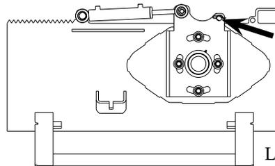
STEP 2: Raise the Hammer approximately two feet (2') off the ground with the Hammer tilted slightly forward so the grapple jaws are visible.
