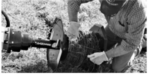
STEP 8: Apply down pressure to insert wire winder spike fully into the ground, compressing the wire winder upper and lower spool assemblies and relieving pressure on retention pin.
