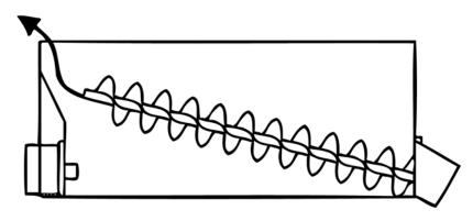
STEP 7: Place the auger on a secure work platform. Use a hammer and chisel to remove the lock nuts from the flights to be replaced.
