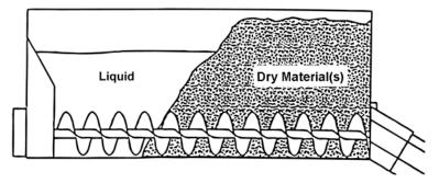
STEP 2: Run the auger in reverse. This will draw the dry material(s) into the liquid and up the motor end of the bucket. The mixture will roll back into the mixing material(s).
